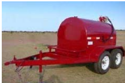
Example of double walled fuel storage trailer
